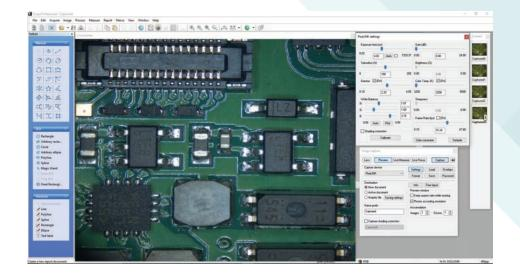
Live Measurement and Overlay Settings - Users can perform measurements on the live preview image, using the crosshair or grid masks to center and count. The grid masks include calibration data. Calibration marker (scale bar) can be placed on the live preview image. The marker (scale bar) can also be burned on each captured image automatically. Any standard file format image can be chosen to see it above live preview image.
